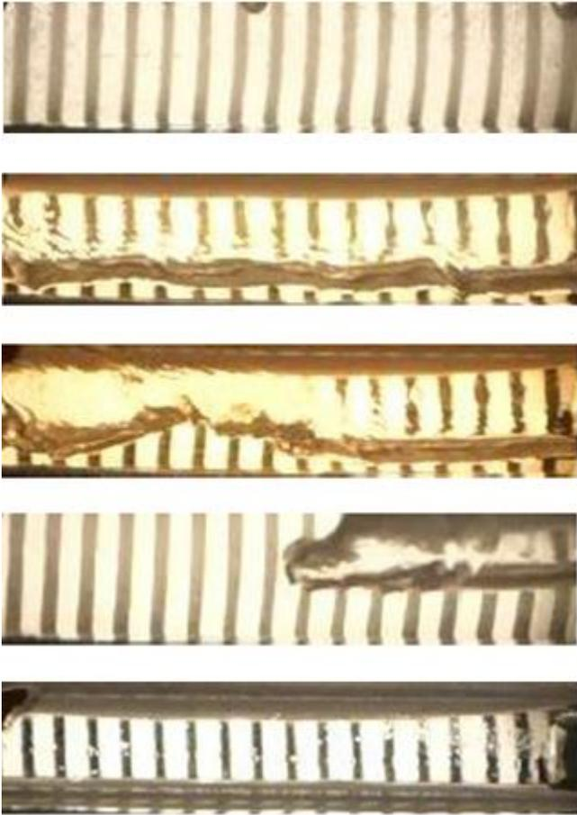
Figure 9: Camera observed flow patterns (complete fluid; stratified; wavy stratified; elongated bubble; annular) [1]
